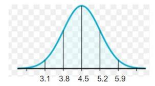
The graph shows 2 standard deviations below and above the mean. Within these two end values (3.1 and 5.9), there will be 95% of the data values.
